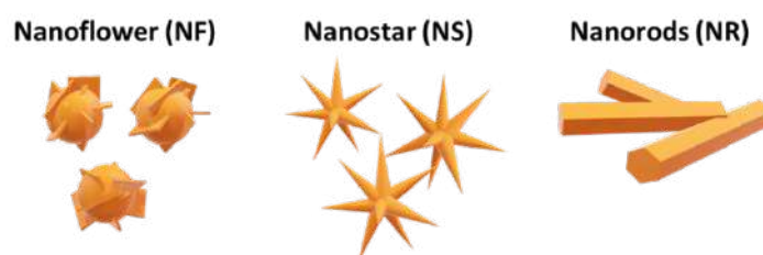
Figure 1. Schematic illustration of the ZnO nanostructures with various morphology synthesized by varying hydrothermal synthesis condition.
